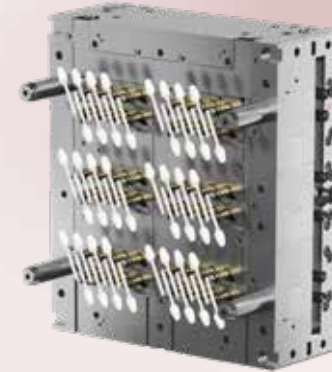
Part weight: 1.32 g Part thickness: 0.7 mm System type: 48 drops system Tp series Injection type: Cylindrical valve gate
